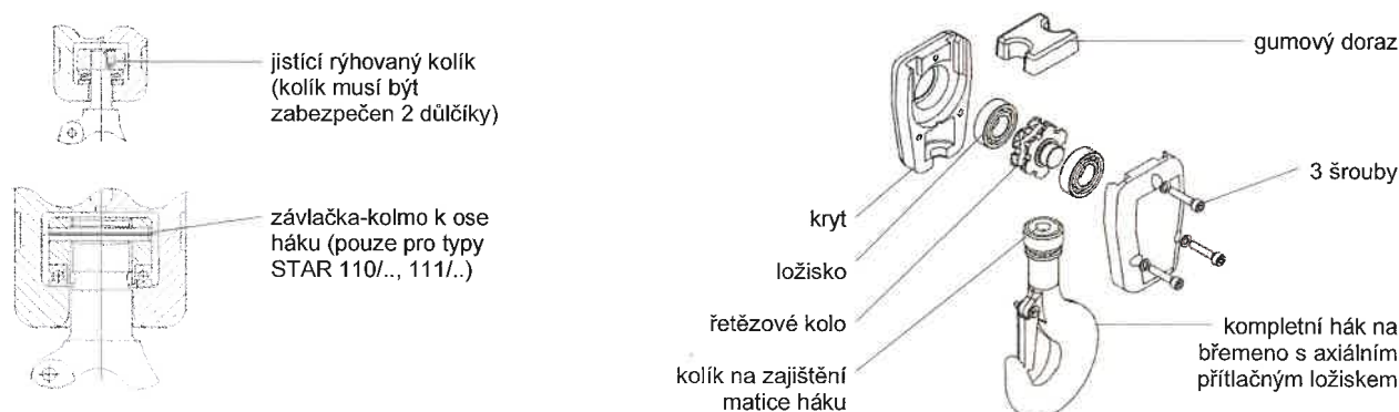
Obr 5: detail kladnice
